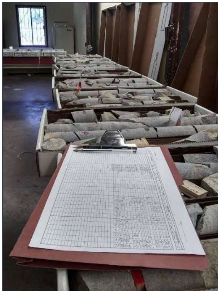
Figure 8.2: Example of a Logged and Sampled Drill Hole
