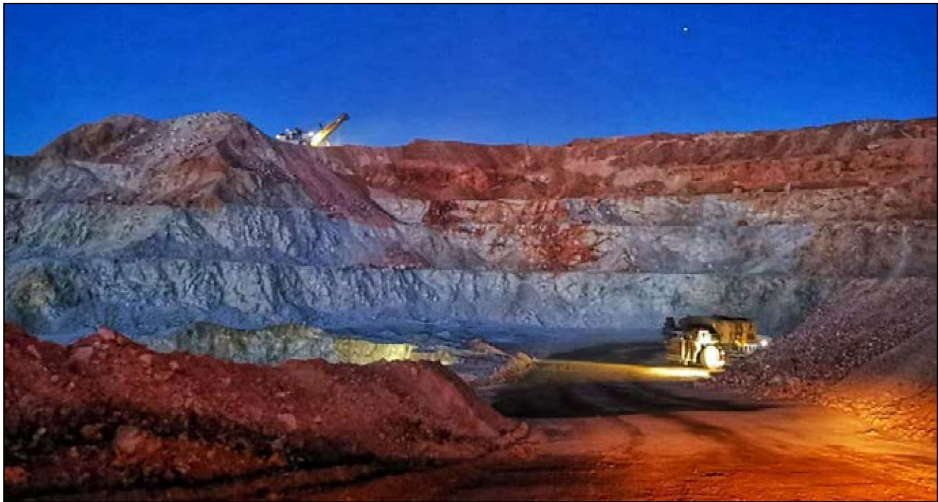
Figure 6.8: Oxidation Zone (Red) and Supergene Zone (White) in the Western Part of the La Caridad Pit
