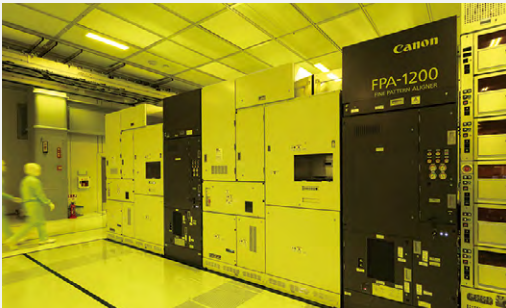
Nanoimprint lithography equipment being used for mass production verification at KIOXIA Corporation
