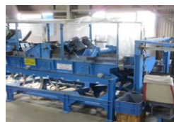
▲Aluminum sorting by continuous mixed metal sorting machine
