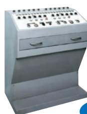
1963 OSP III World’s first absolute-position encoding system NC
