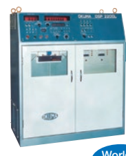
1972 OSP2000 World’s first commercial CNC
